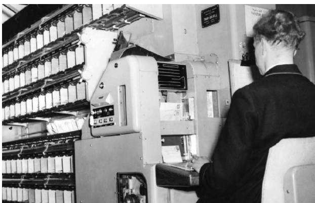
Figure 4. Medical Research Council Applied Psychology Unit research in the Post Office. In the early 1960s mechanisation of letter-sorting envisaged a keyboard operator copying postcodes to enable mail to be sorted electronically, as illustrated (source: Reynolds and Tansey 2003).
