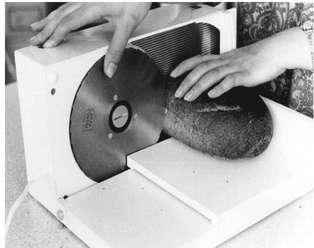
Figure 1. Faulty position of on-off switch on electric bread cutter. The position of the on-off switch leads to serious risk of slicing the right thumb.
