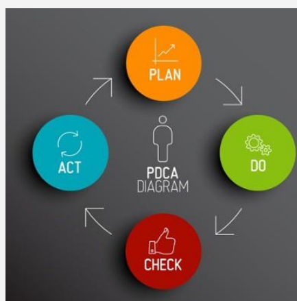
Fig. 1 - Layout of the "Plan-Do-Check-Act" methodology– PDCA. The PDCA cycle is a way to achieve continuous improvement in business, development and production processes. In the same way that a circle has no beginning or end, so is the constant and uninterrupted PDCA approach.
